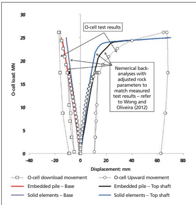
Figure 7. Back-analysis results compared with O-cell test results of one of the test piles
