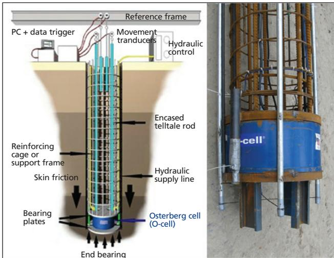
Figure 6. O-cell testing arrangement for prototype test piles
