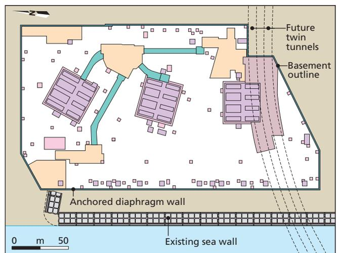
Figure 4. Barangaroo South basement B2 plan showing perimeter diaphragm wall and transfer structure over future Sydney Metro tunnels
