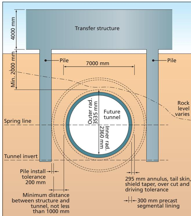
Figure 10. Typical cross-section of transfer structure over the future Sydney Metro tunnel (dimensions in mm)
