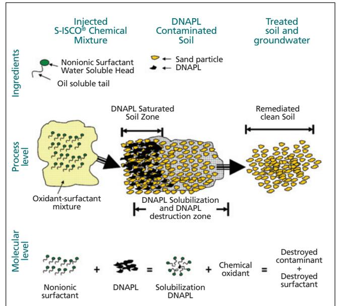
Figure 3. Surfactant-enhanced in-situ chemical oxidation contamination remediation process. DNAPL, <AQ4>
