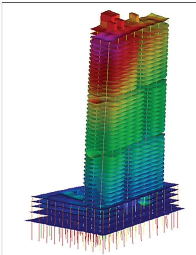
Figure 12. Example of commercial tower finite-element framing model and analysis results
