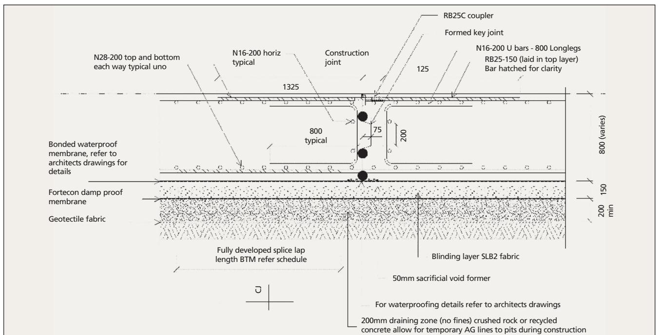
Figure 9. Typical basement slab construction joint showing proposed splicing and waterproofing details
