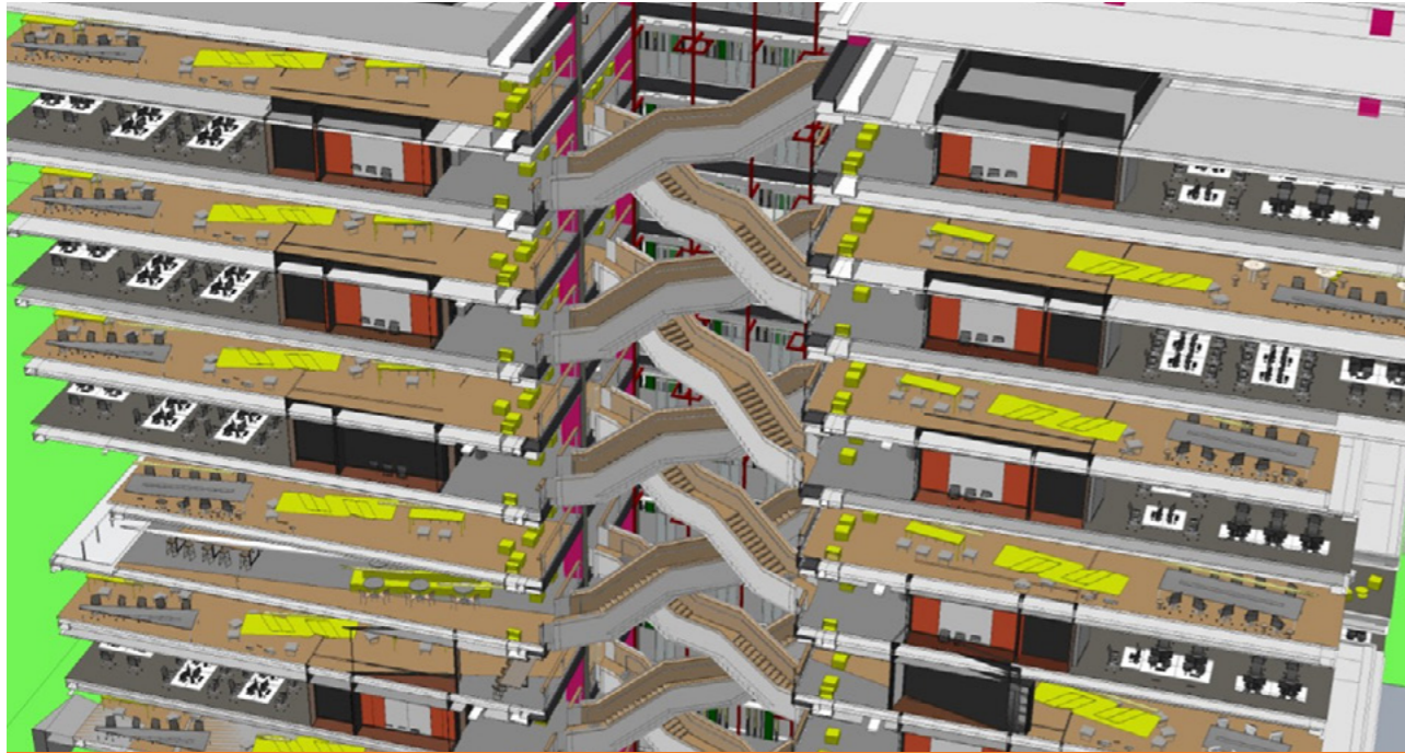
3D modelling of stair installation at 3PS
