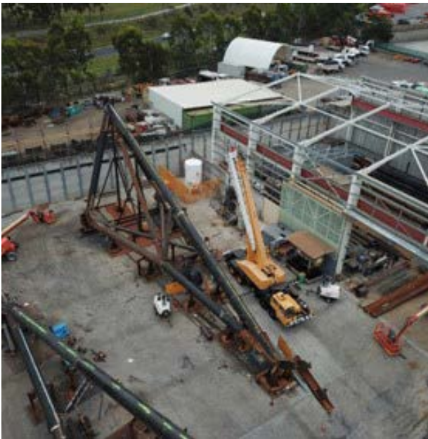
Dry fit of Derrick in the manufacturing yard, positioned in Jig, checked for dimensional conformance, prior to initial welding
